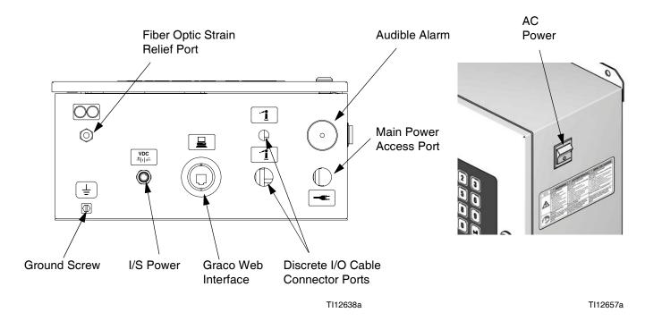
Fig. 6. EasyKey Connections and AC Power Switch
